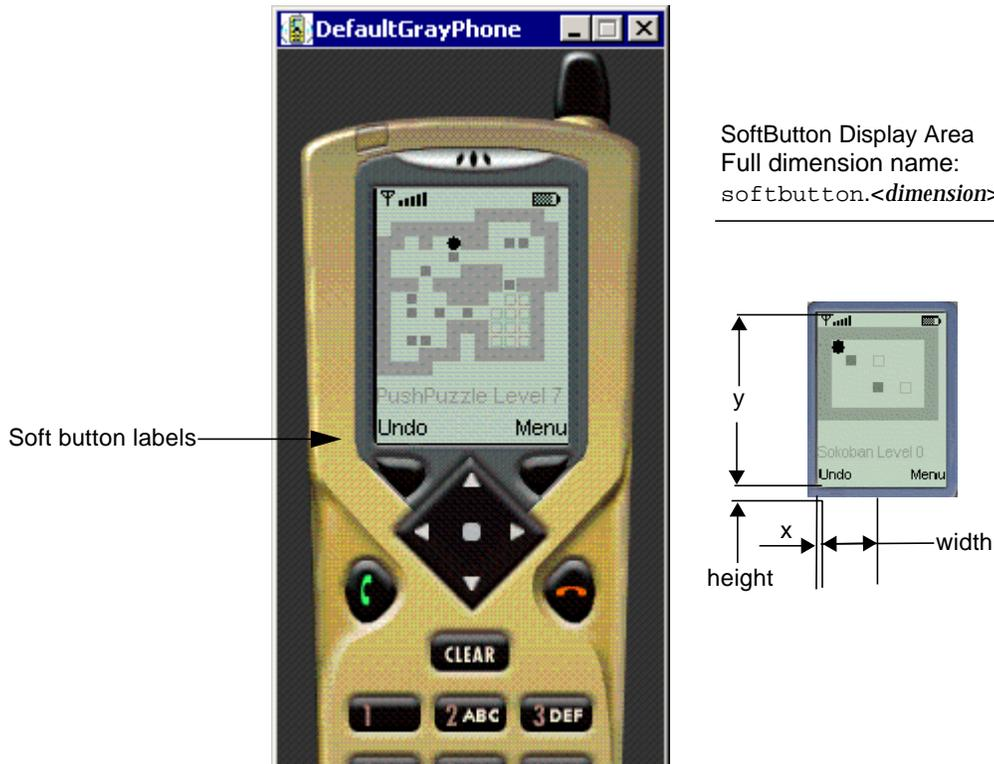
**FIGURE 3** Soft Button Label Areas on the Emulated Device Display
