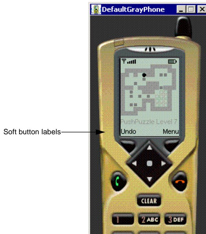
**FIGURE 7** Soft Button Labels on the Emulated Device Display
